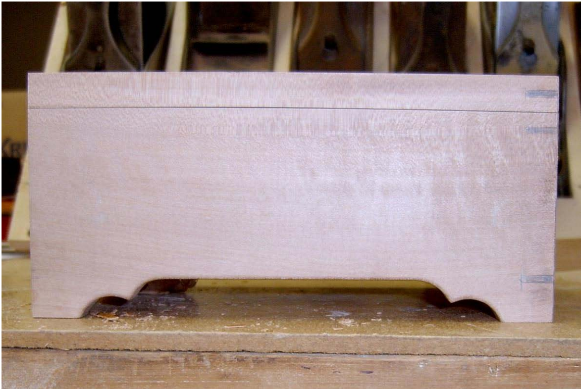
Here I have laid out where I want my keys to go. I do this after I cut the lid free to make sure I get the keys centered on the lid.
