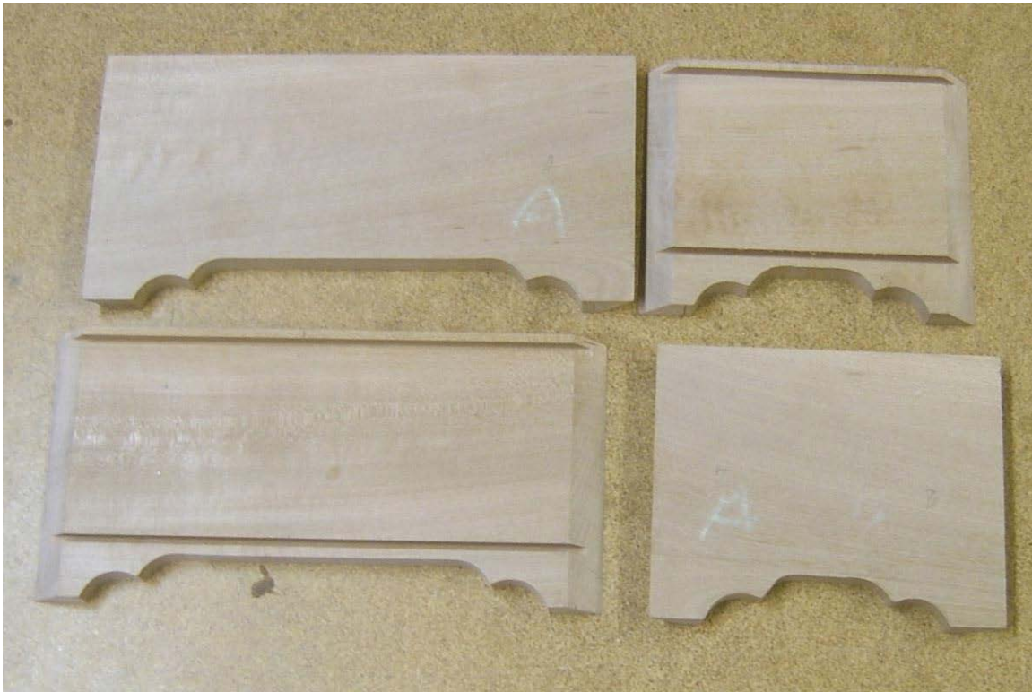
Here are the feet after routing.
