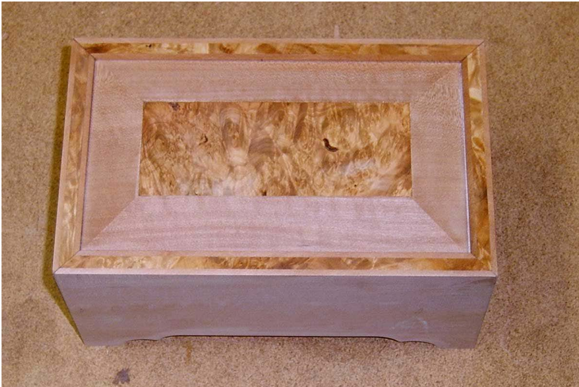
Here is how the top panel looks with a bit of mineral spirits on it. You can see the flat spots on the lower left side and on the bottom right side.
