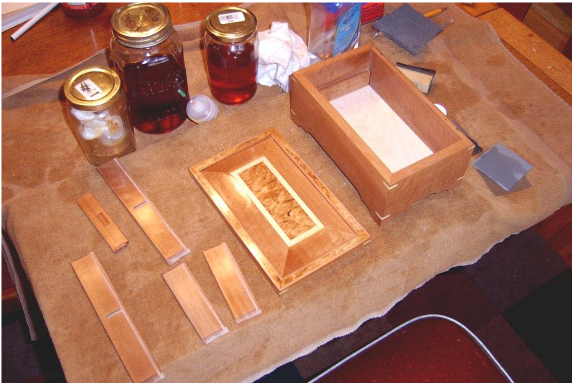
Here is my setup to do my French polishing. I have one and two pound cuts of shellac, denatured alcohol, mineral oil, a small rubber, a couple of squeeze bottles to drip shellac on the rubber with, some 300 and 2500 grit sandpaper for repairs, a small sanding block, a grey Scotch-Brite, and my soft rag. And that is as much as I will tell you about how I French polish as I am still very much the amateur at it. After shellacking, I will glue the top and bottom together and then wax the whole thing using a white Scotch-Brite pad.
