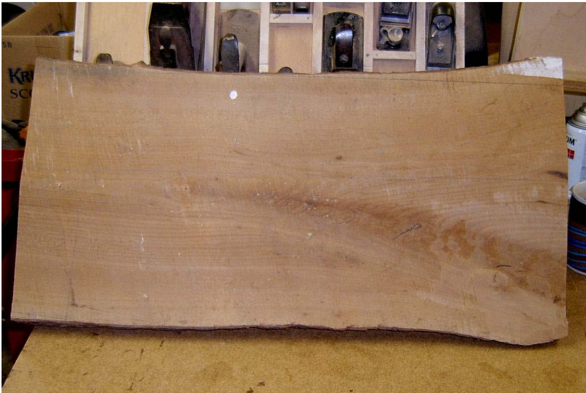
This is the beginning piece of Madrone. Air dried for over 25 years. It is about 24" long, 12" wide & 5/4" thick. You can see what I am trying to get out of it marked in pencil.
