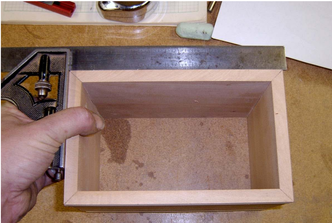
Miters complete and box is squared. The small gaps at the miters are from a dull blade and will be closed when the fuzz is removed.
