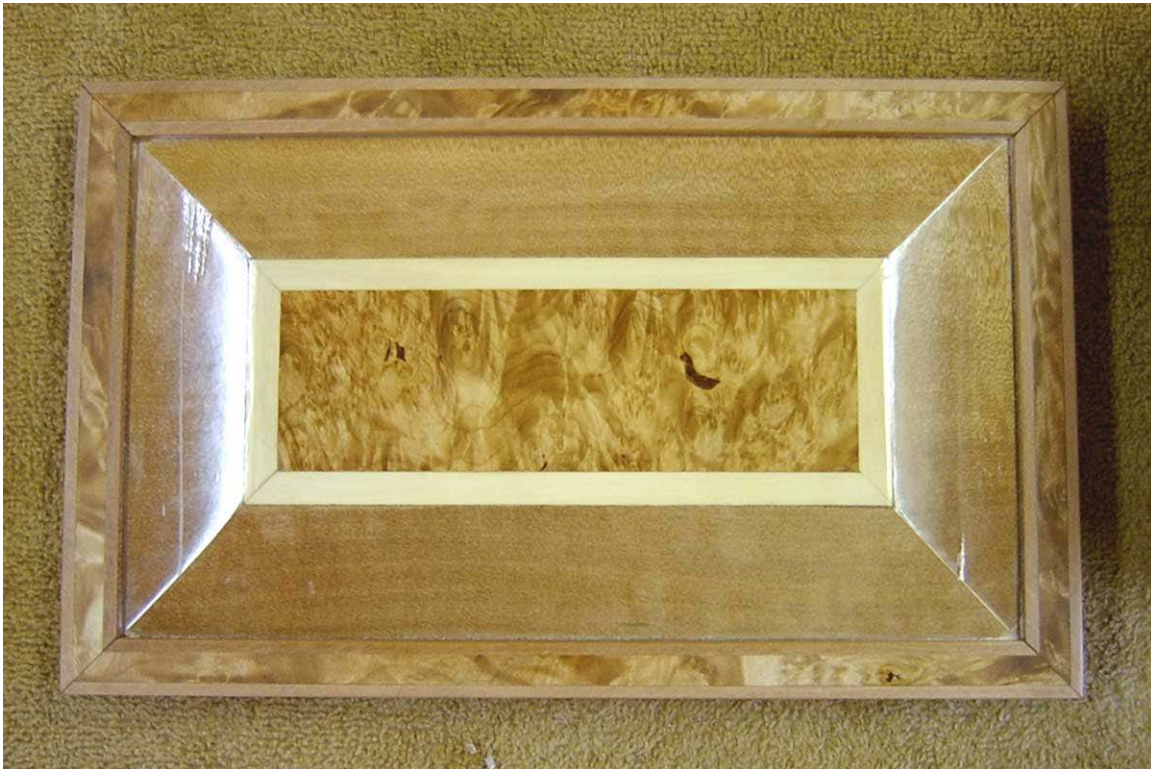
Here I show the top panel after oiling. You can see the box must not have been tight in the vice when I was flushing the sides and dented the top. SOAB! A lot of it will come out when I do the final shellacking but I just brought the quality of the box down several notches for sure.
