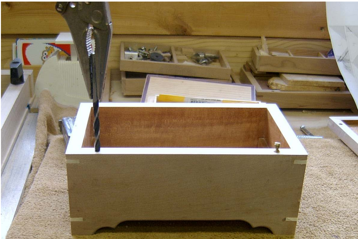
I now need to fit up the hinges. I test fit the hinge and if the hole isn't deep enough, I use my 5mm bit to deepen them by hand. I don't use the drill press when doing this as I can be a lot more accurate this way. If the hole is too deep, use a small piece to dowel to fill the hole.
