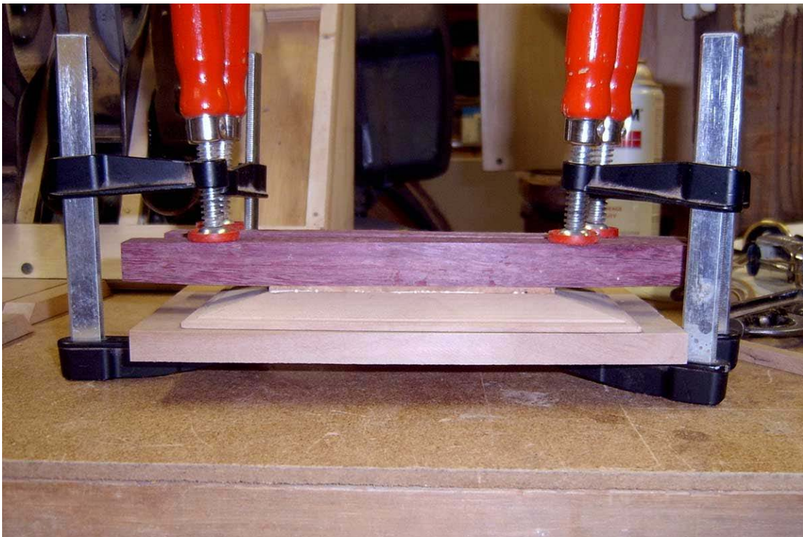
All clamped up with small cauls to help get good pressure.
