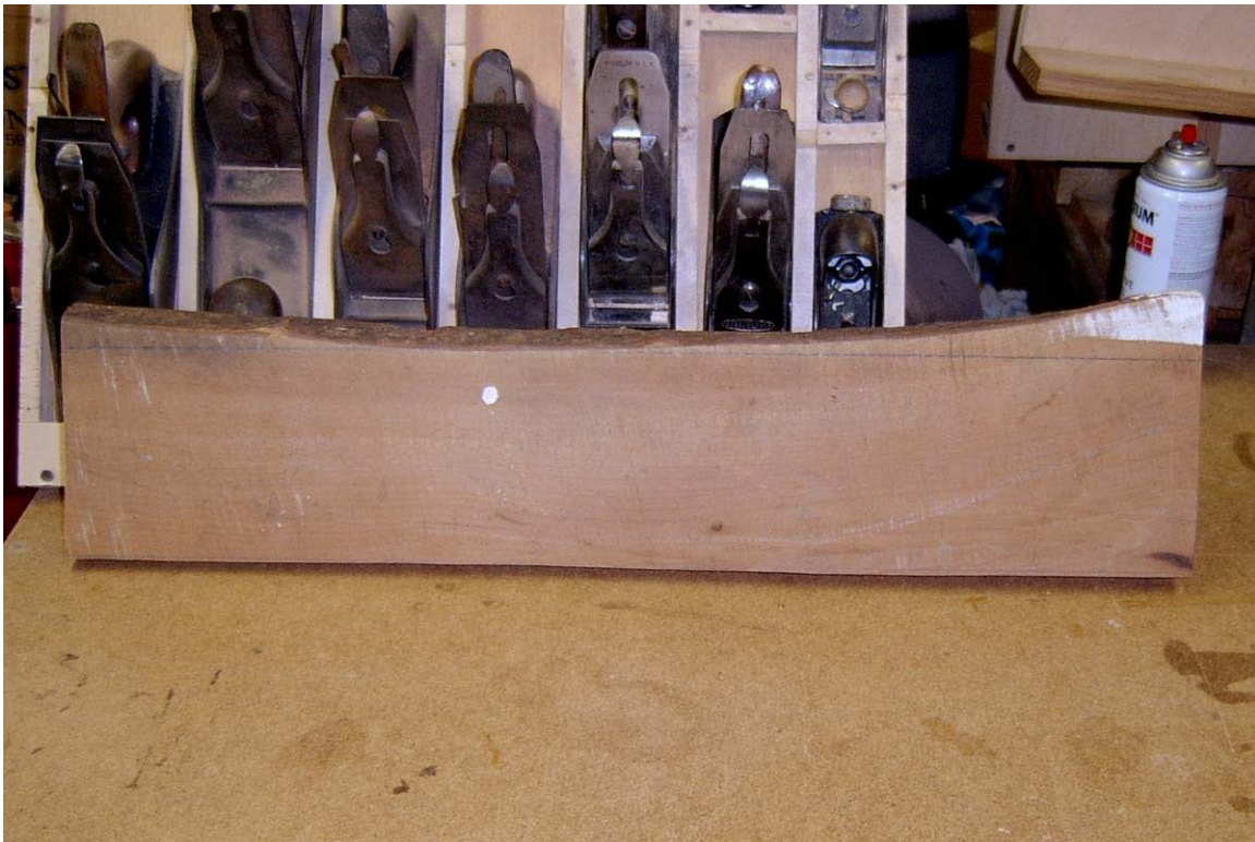
Piece after being roughed ripped to width on the band saw.
