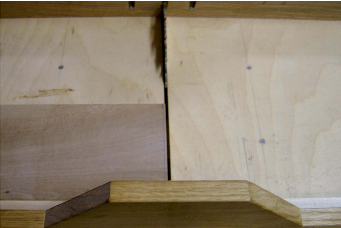
Here I show trimming the ends square to the sides.
